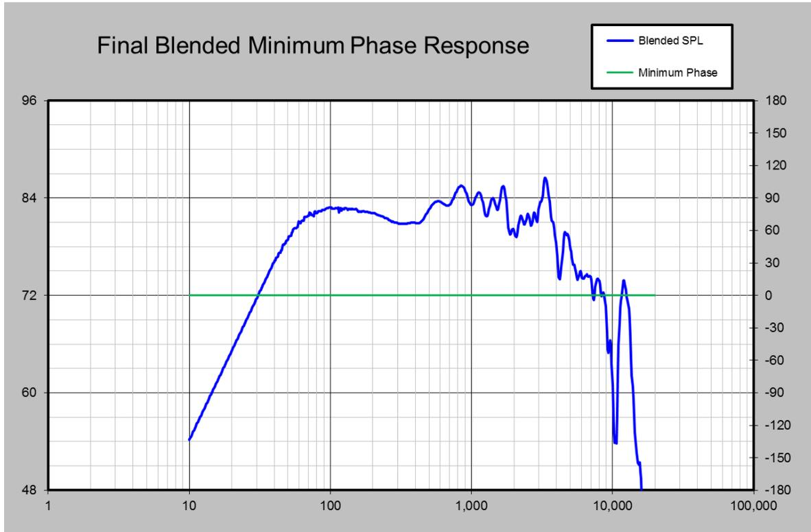
This graph is representative of most spliced graphs and matches what we will see in most tutorials and manuals on splicing near-field and far-field data. However, there is a problem with this data and it is right in the region that is most critical to us – in the 150-200 Hz region.
