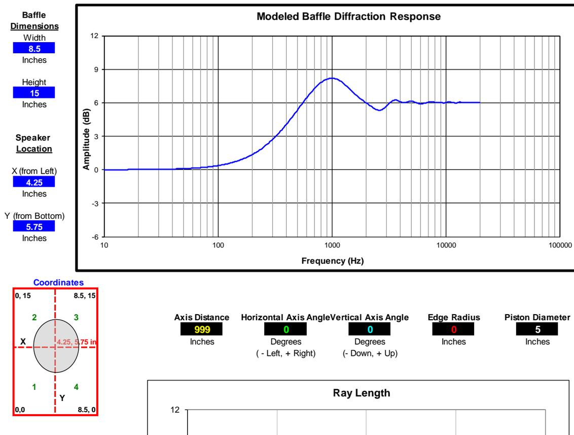
When this curve is added to the near-field response it can be overlaid with the far-field data more effectively because now both near-field and far-field response data include the baffle step information in the critical range where they overlap.
