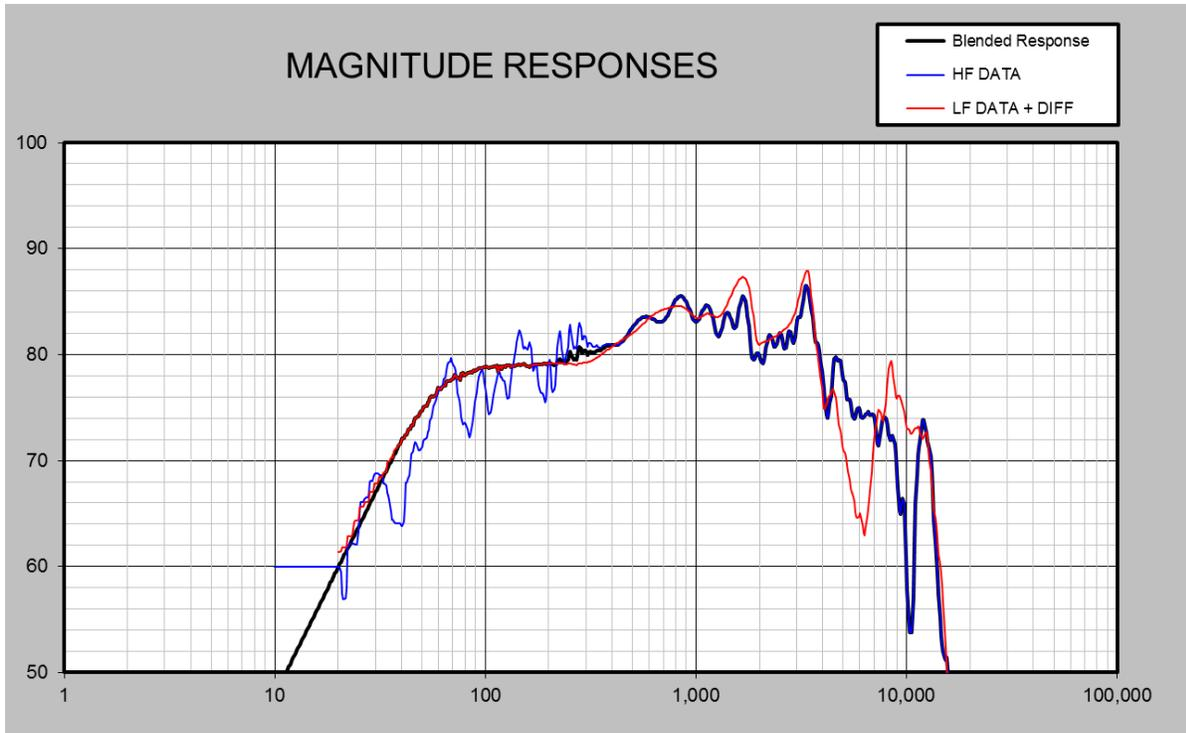
The near-field plus diffraction even aligns well with the blended far-field in the data below 30Hz as well.
