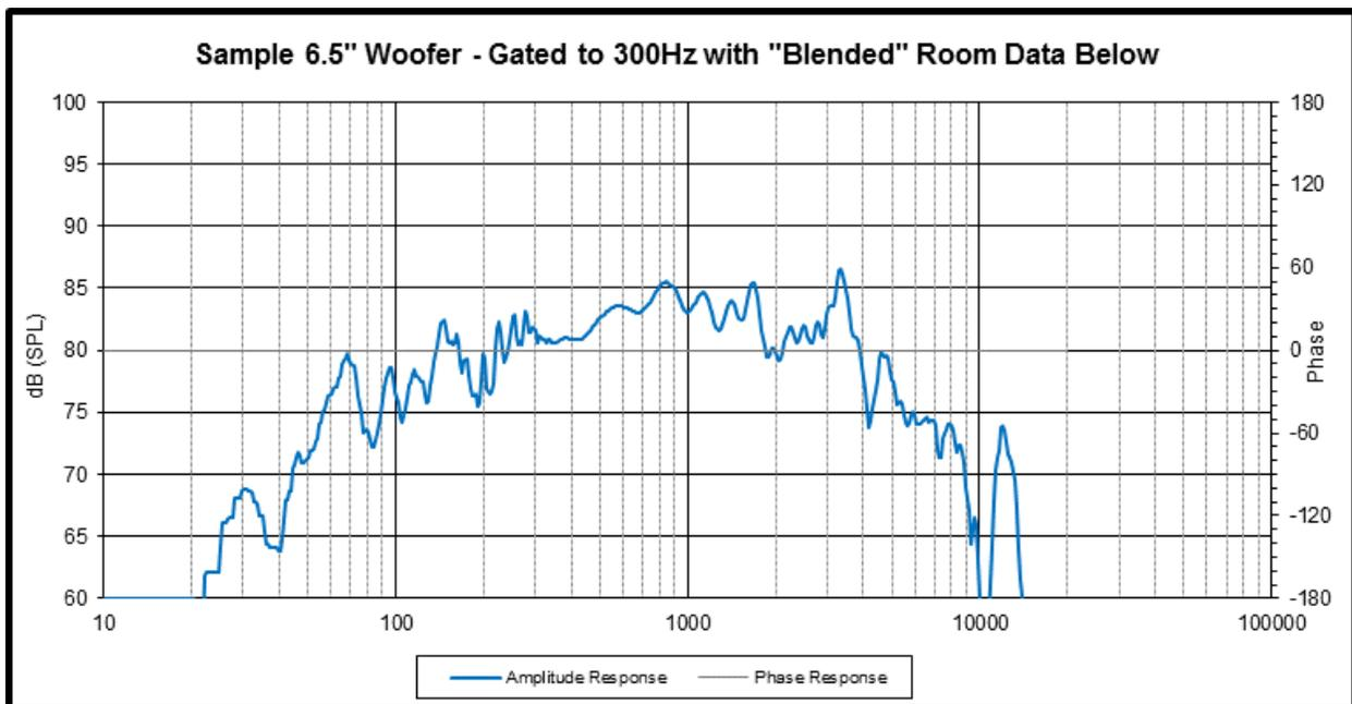
In this graph the gated impulse response is good down to 300 Hz and the response below 300Hz is blended with the room response data. The Omnimic was used to measure this response.
