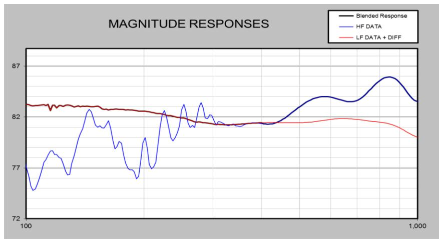
Using 400 Hz as our splicing point, which is the traditional method, yields the following merged response plot (I have not extracted minimum phase yet, so the phase data does not show):
