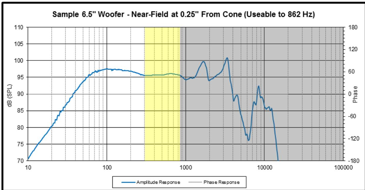
The merging or slicing of the near-field and far-field responses need to take place in the yellow frequency band that is shared by both sets of data, at a point where we can line up both sets of data together.
