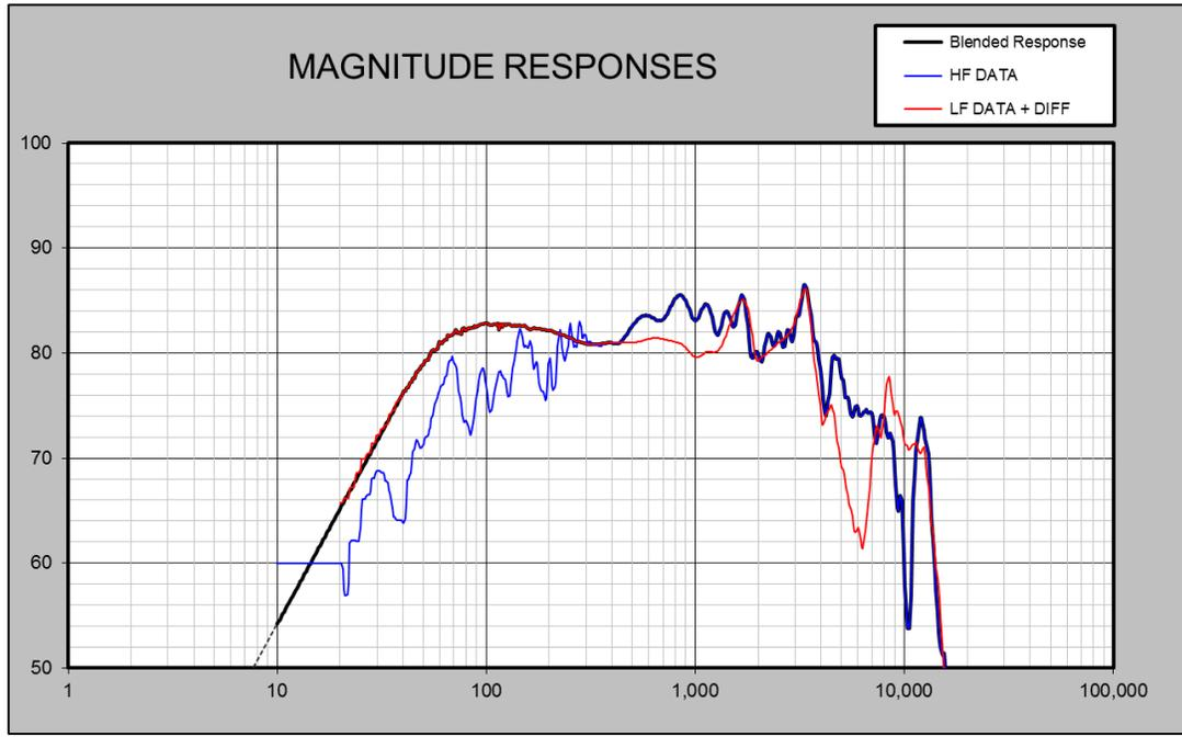
The red line is the near-field measurement and the thin blue line is the far-field measurement. Zooming-in we see that we can line-up both responses in the region between 300 – 450 Hz. This is very typical, and the normal range you will find for splicing data.
