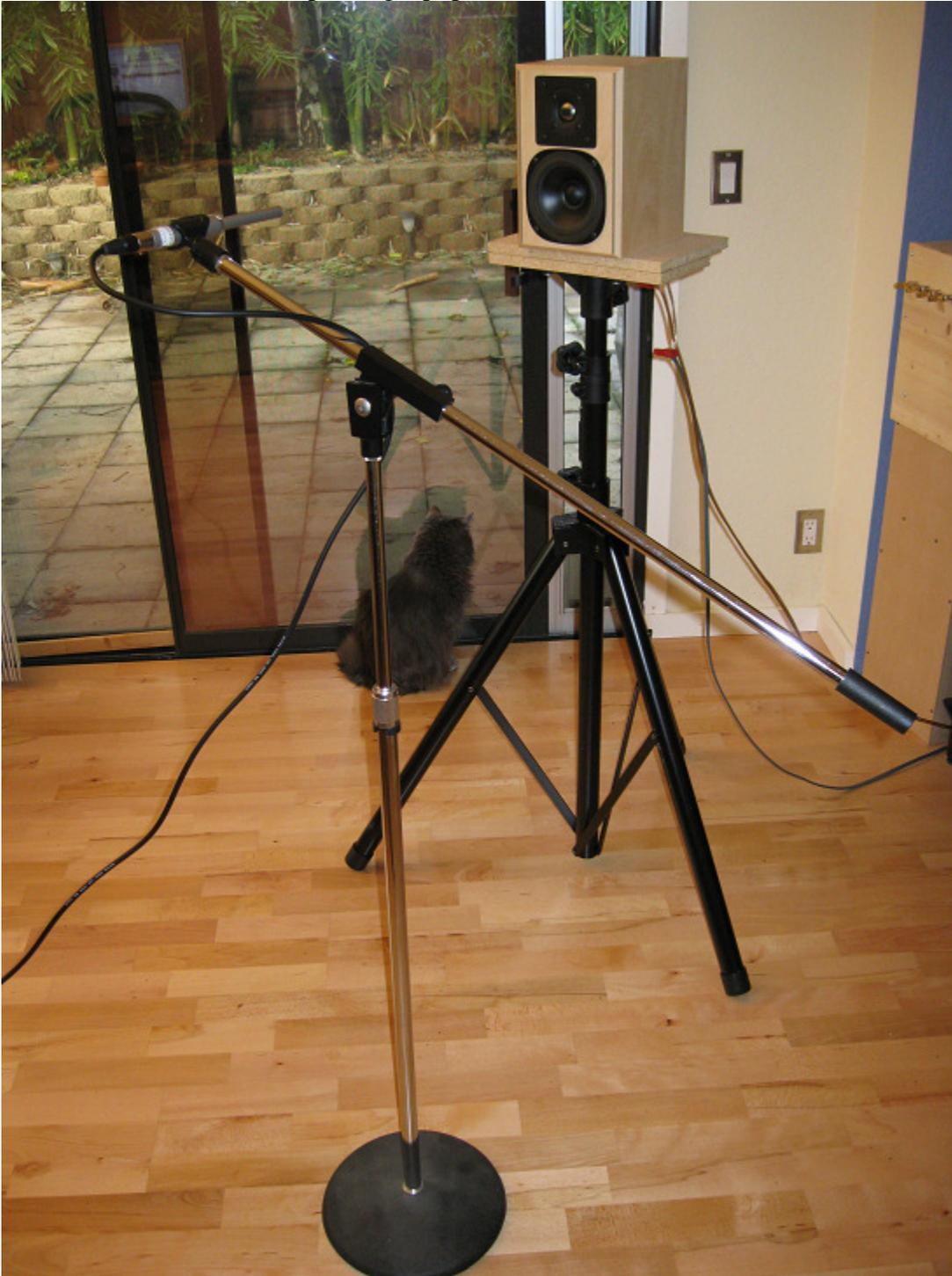
This is a small room (10' x 12') with a 7' ceiling. In a larger room I would position the speaker near the middle of the room and farther above the floor if the ceiling is higher. The mic is on axis, about 30 inches away from the speaker. This is about as close as I would position it, since you want to be away from the near-field.
